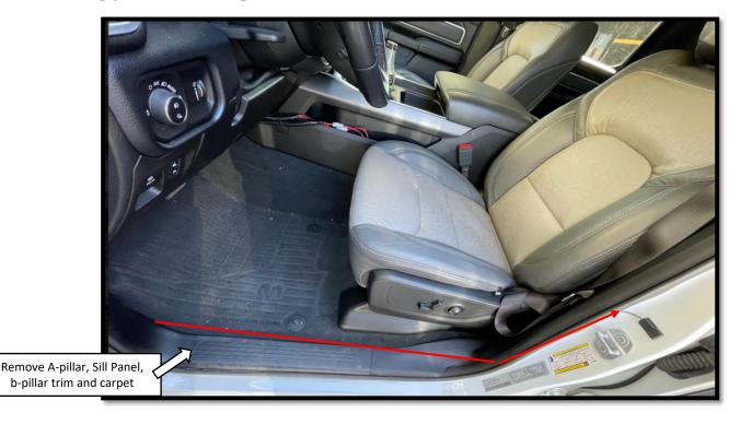
**Step 14:** Route the Driver side door trigger wire (brown) towards the Driver side b-pillar. Route the Passenger side door trigger wire (white) under the center console and over to the Passenger side b-pillar. Route the black disable switch wires to the center console.
