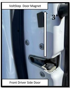
**Step 17:** With the front driver side sensor attached, you can determine the correct position for the door magnet. peel the backing from the double-sided tape and stick the magnet on the door. Align the bottom of the magnet with the 3"
