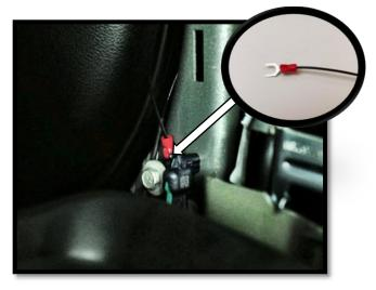
**Step 15:** The door trigger sensor harness will need a ground connection to the vehicle. Locate the hex head screw near the seatbelt assembly and install the ground under the plastic housing as shown.
