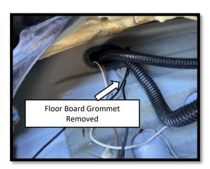
**Step 13:** On the driver side, remove the front kick panel, front door sill trim panel, b-pillar trim panel and pull the front driver carpet back. Now go under the truck and locate the plastic grommet on the driver side floor board. Drilla 7/16" hole as shown. Make sure not to drill through the carpet.
