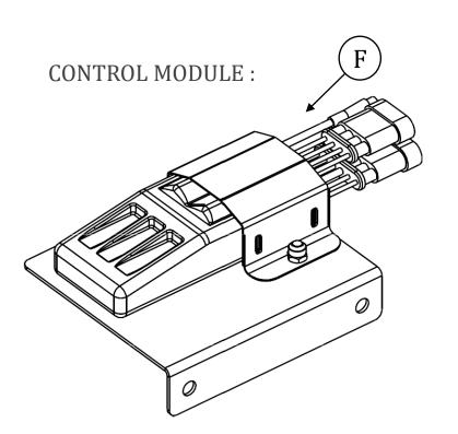
Notice: As shown in the picture, there is a four conductor plug, a six-conductor plug, a black two conductor plug, and a red two-conductor plug.
