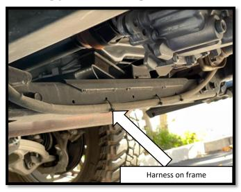
**Step 12**: Route the motor wire harness from the controller to the Passenger side frame rail of the vehicle. When routing the harness keep clear from any moving parts and avoid direct contact with the exhaust system.
