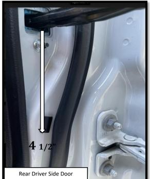
**Step 19:** With the rear driver side sensor attached, you can determine the correct position for the door magnet. peel the backing from the double-sided tape and stick the magnet on the door. Align the bottom of the magnet with the 4 1/2"
