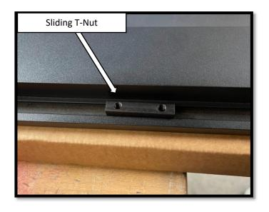
**Step 7:** Install the Driver side running board. With assistance, begin by positioning the board on the front and rear motor assembly bases. Align the sliding T-Nut on the running board with the slots on the front and rear motor base. Once the T-Nuts are aligned, rotate the running board so that the T-Nuts set in the slots on the base of the arms. Repeat Steps 3-6 to install the motor linkage assemblies and running board on the Passenger side.
