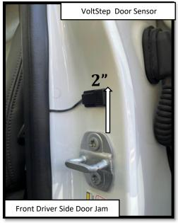
**Step 16:** FRONT DOOR: With the weatherstrip peeled back, route the sensor wire underneath it. Clean the surface by cleaning with a 50/50 mix of isopropyl alcohol and water or equivalent. Once the surface is completely dry, peel the backing from the double-sided tape and stick the sensor on the door jamb. Align the top of the sensor with the 2"
