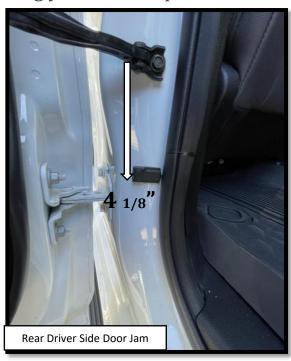
**Step 18:** REAR DOOR: With the weatherstrip peeled back, route the sensor wire underneath it. Clean the surface by cleaning with a 50/50 mix of isopropyl alcohol and water or equivalent. Once the surface is completely dry, peel the backing from the double-sided tape and stick the sensor on the door jamb. Align the top of the sensor with the 4 1/8"
