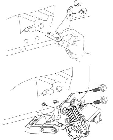
**Step 3**: Install the Front Driver side motor using (1) Nut Plate , (2) M8 Hex Bolts. Holes that do not have factory threaded inserts will require the threaded nut bracket that is included in this kit. The hardware should be hand tightened only until snug. This will allow the motor assembly to move and align easier when installing the running board.
